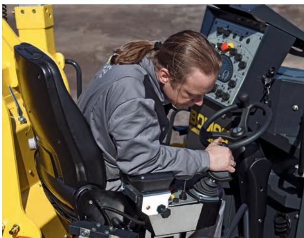
The swivel seat, which can be swivelled 45 degrees, provides the best view of the loading truck and milling edge.
