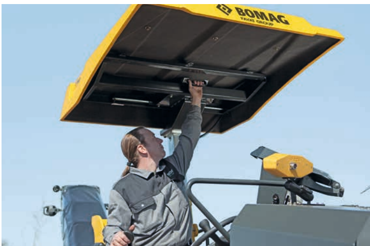
The roof can be easily shifted laterally; perfect for confined site conditions.
