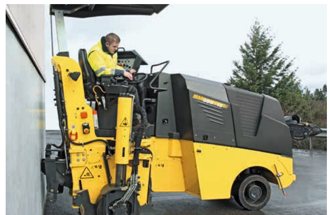
No control cylinder affecting the rear area of the planer.
