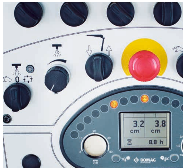
Water spraying can be controlled easily using two control switches.
