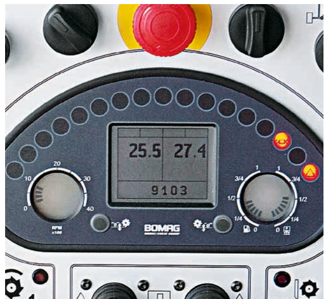
The digital milling depth indicator and the switches for the traversing speed are directly in the operator's field of vision.
