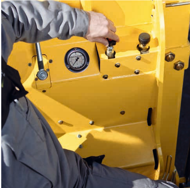
Convenience while seated – adjusting the scraper pressure.
