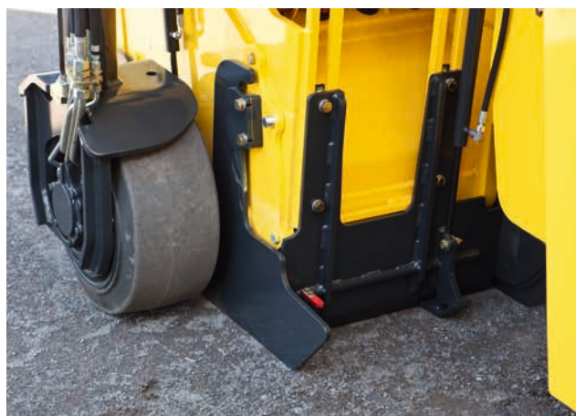
Hard metal grade shoes – they can withstand a lot of wear.
