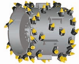
Quick-change milling drum Milling width: 600 mm Line spacing: 15 mm Milling depth: 0-210 mm
