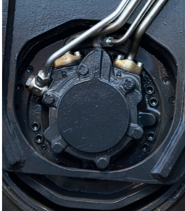
Installation of the hydraulic lines close within the gear housing.
