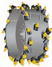
Quick-change milling drum Milling width: 300 mm Line spacing: 14 mm Milling depth: 0-160 mm
