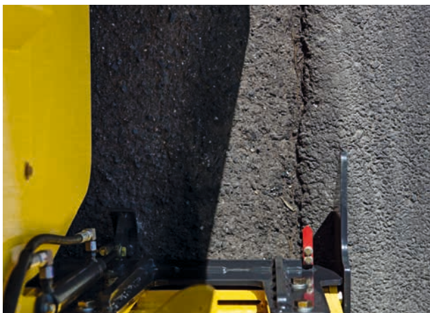
Accurate positioning is enabled by the milling edge indicator on the retainer.
