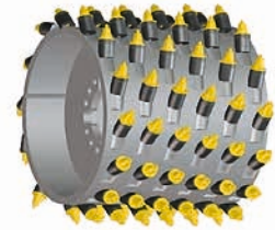
Quick-change fine milling drum Milling width: 600 mm Line spacing: 6 mm Milling depth: 0-50 mm
