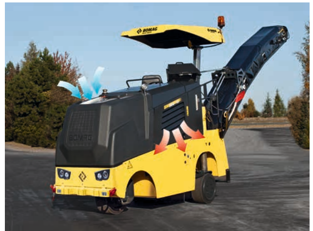
Sound insulation and intelligent air duct.
