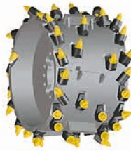
Quick-change milling drum Milling width: 400 mm Line spacing: 14 mm Milling depth: 0-160 mm
