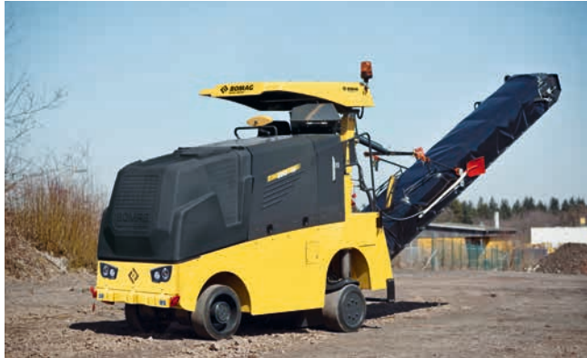
The large, optional weather protection roof can be height adjusted from the seat without interrupting work.
